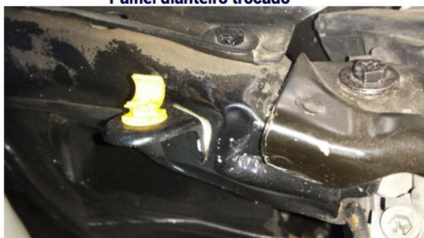
Ponta do painel frontal amassada
